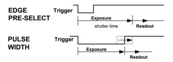
Fig. 6. External trigger modes
